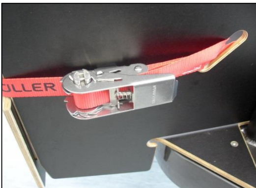
fig. 8: tightening the tensioning belt
